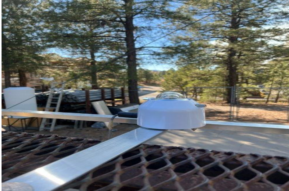
Figure 24: Pyranometer Mounted on Crossbar
