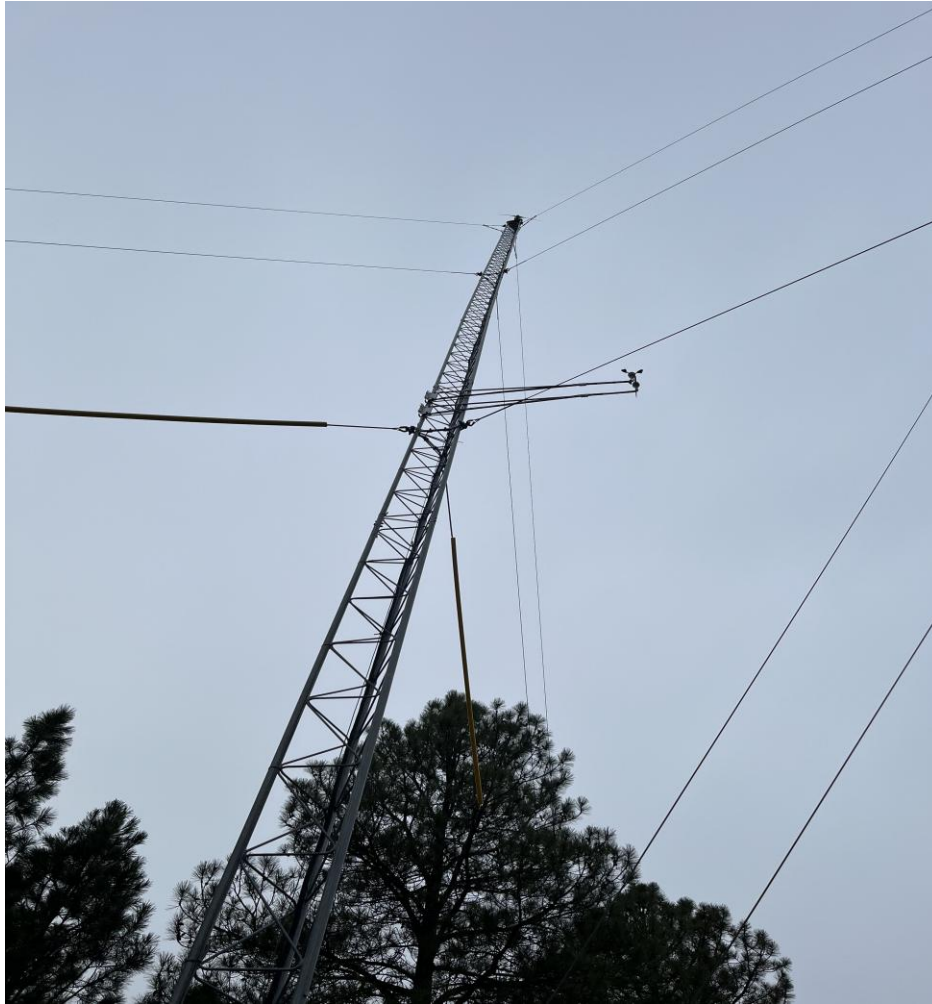
Figure 26: Anemometer and Wind Vane Mounted at 30ft
