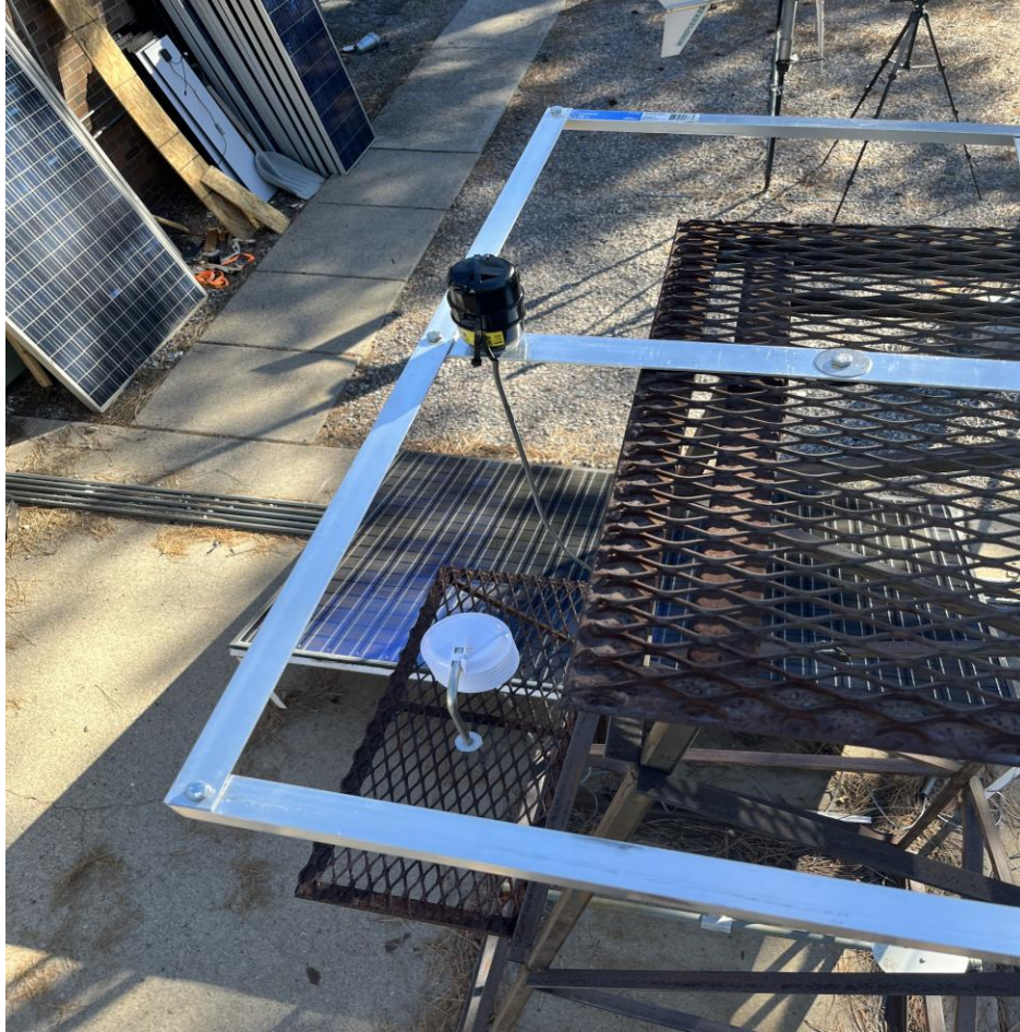
Figure 25: Mounted Barometric Pressure (top) and Temperature Sensor (bottom)
